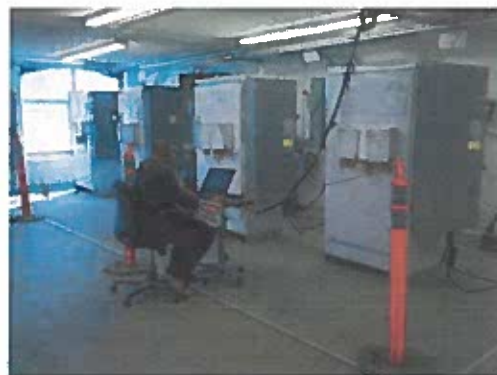
8 Hour HASS Burn-in Test and Final Verification
